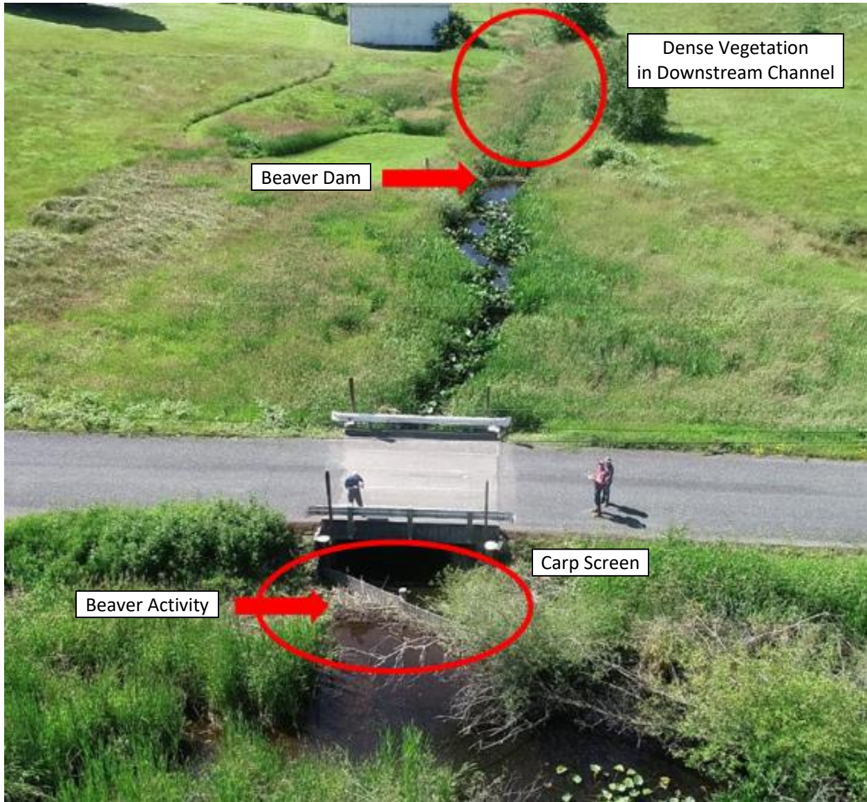
Figure 4 – Features likely affecting outlet channel capacity and therefore lake levels (Photo taken June 17, 2021)
